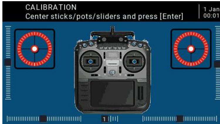
D. The third move all the gimbals, knobs, and side sliders of to their respective maximum and minimum positions. The system will record the maximum and minimum values. At this time, 6POS (six position button) may be pressed one by one. The system records the value of each button. The value of the key can be viewed at the bottom of the page. After all the above steps are completed, press Enter key to complete the calibration, and the system automatically returns to the previous page.
