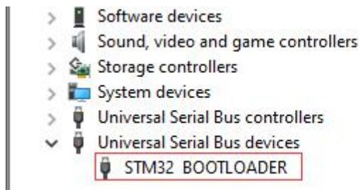
Before writing the firmware for the first time, you need to replace the STM32 BOOTLOADER driver to ensure that the OpenTX Companion software can recognize this hardware type and write the firmware correctly. The replacement method is as follows:
