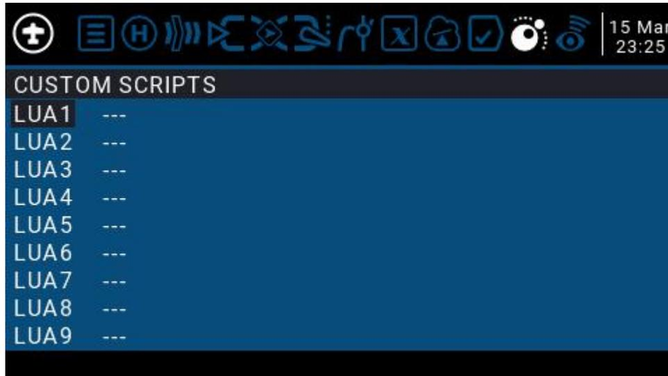
“The Custom Scripts page is for mixed-type scripts that run continuously. These scripts should be placed in the / SCRIPTS / MIXE / folder of the SD card.
