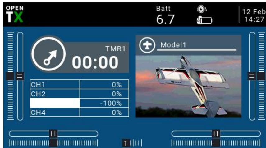
**Top menu bar:** The default top menu bar displays speaker volume, remote control battery level, receiver signal strength (RSSI), and time and date. Batt is a custom top display remote control voltage; users can also add other display information and widgets.
