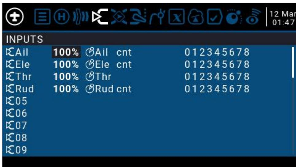
To set an entry, press and hold the ENT key on the current entry and a submenu will pop up
