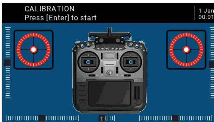
C. In the second step, place all the gimbals, knobs, and side sliders in the middle position. The system obtains the midpoint value, and then press the confirmation key to continue to the next step.
