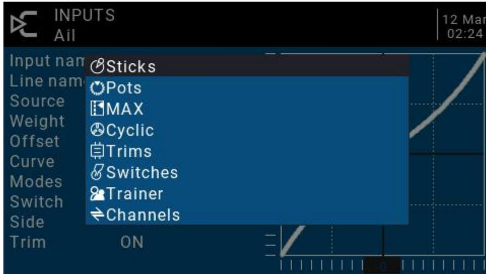
Weight: Normal range is a value between  $\pm 100\%$  will be zoomed to the gimbal operation. If you enter a negative value, for example  $-100\%$  means reverse the output. Note that channel inversion should not use negative values on the Inputs page, and to reverse channels should be reversed on the Outputs page.
