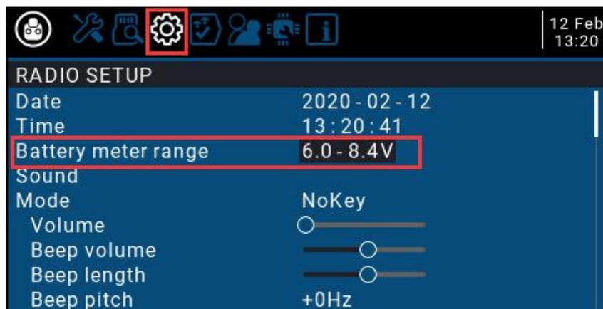
B. On the current page, turn the scroll wheel to find Battery low (low voltage alarm), and fill in the alarm voltage as shown below. When the remote-control voltage is lower than the current set voltage, the system will play a voice alert and report that the battery voltage is low.
