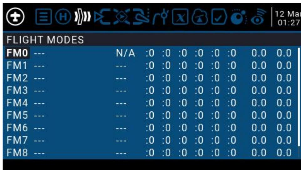
There are 8 flight modes plus the default FM0 available. The first item of FM1-FM8 requires a trigger switch. When no switch is on, FM0 is enabled by default.
