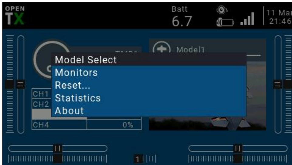
Select to enter the model selection page, which is used to select, create, switch, delete and copy models.
