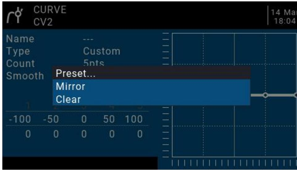
**Preset:** Select presets with slopes of  $-45^\circ$ ,  $-33^\circ$ ,  $-22^\circ$ ,  $-11^\circ$ ,  $0^\circ$ ,  $11^\circ$ ,  $22^\circ$ ,  $33^\circ$ ,  $45^\circ$ . When defining more complex curves, choose reasonable presets Will reduce some steps.
