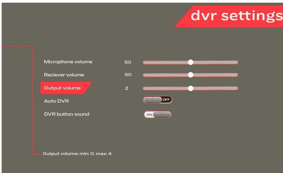
The microphone recording level should be adjusted through the “Microphone Volume” menu. The default level is set to 50%.
