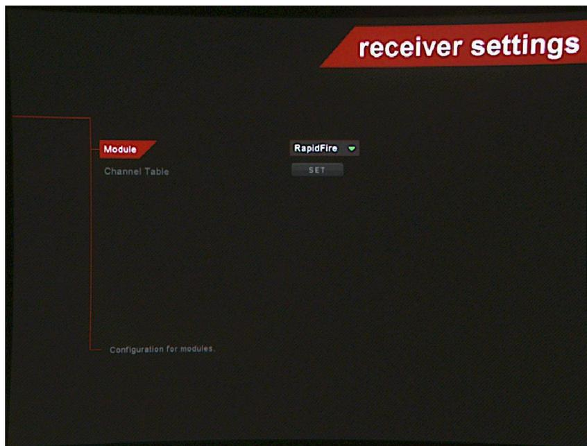
For example, if RapidFire is selected, you will be able to change the channel by short pressing the CHANNEL UP **8** or CHANNEL DOWN **7** buttons on the goggles.
