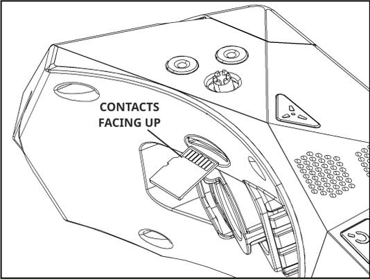
To use the DVR, the micro SD card must be inserted in the dedicated slot in the faceplate.
