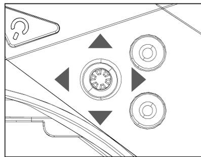
The Left-hand joystick **4** controls the main menu. The main menu incorporates all the main controls and goggles settings.
