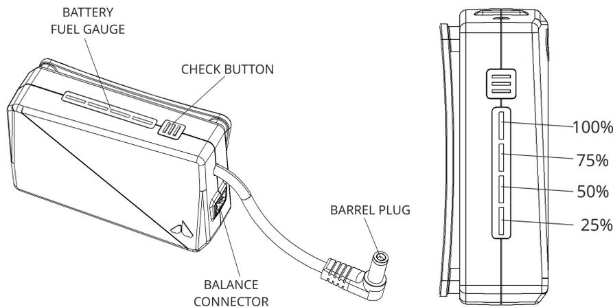
Once the battery is empty, it needs to be recharged. To recharge the battery, connect the barrel plug to the Li-ion battery charger.
