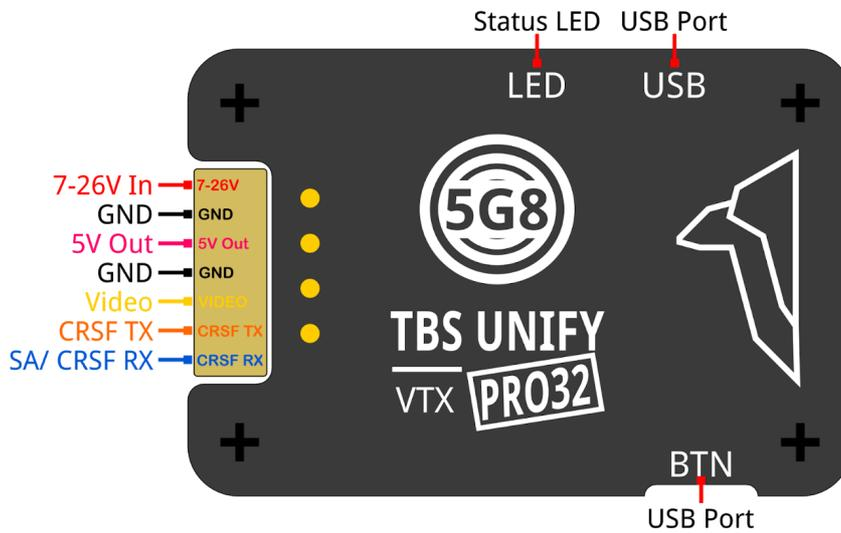
The UNIFY PRO32 5G8 HV comes with a cable assembly with silicon wires for easy installation in your build. There is a filtered 5V output for your camera.
