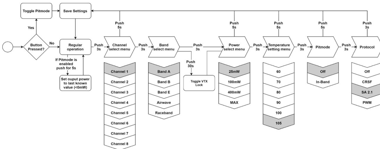
The TBS UNIFY PRO32 5G8 signals selected channel, band and power levels using a startup sequence of LED codes. The same sequence is also repeated in the menu to make it unified. First the **RED** LED flashes to indicate the item being shown. One flash for channel, two flashes for band, three flashes for power level. Subsequently, the **BLUE** LED will indicate the value.
