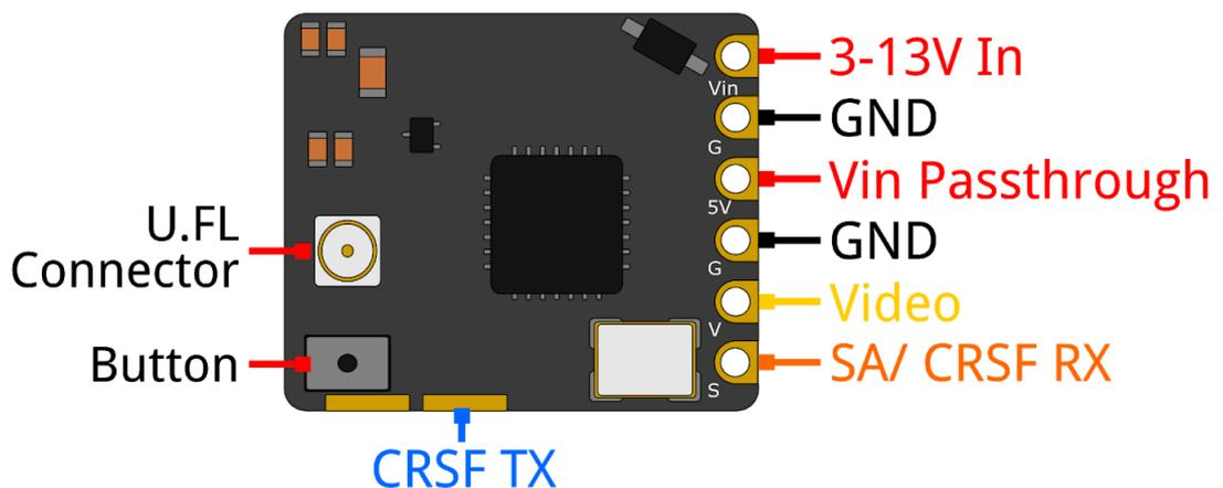
The UNIFY PRO32 5G8 Nano comes with pre installed silicon wires for easy installation in your build. There is a filtered 3-13V input with a pass through output for your camera or other devices.
